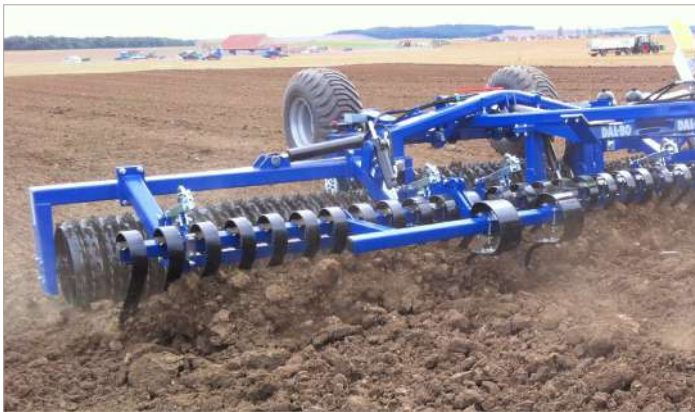
Crackerboard Hydraulically operated cracker board – also fitted with track eradicator tines.100x12 mm.
