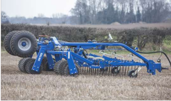
4 row BlackGrass Harrow 6.3m Maxiroll fitted with a BlackGrass harrow of 4 rows of 16mm heavy duty straight tines.werden.
