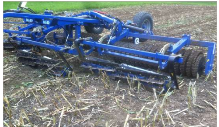
Knife roller Fitted with a 350mm diameter knife roller
