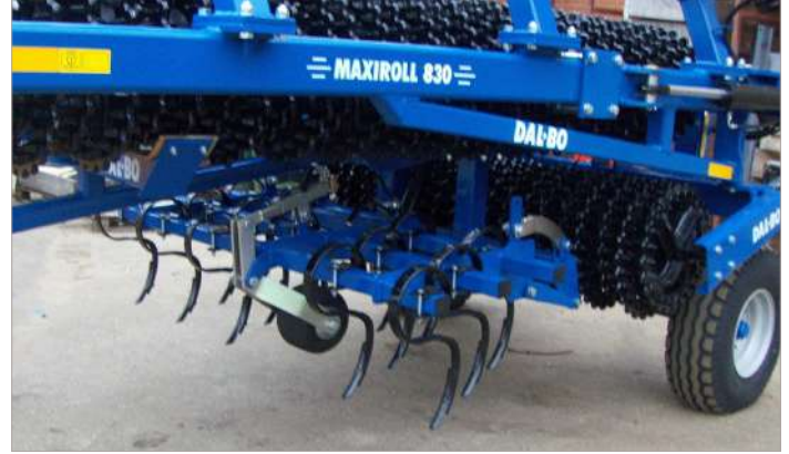
3 rows of H/D spring tines 3 rows of heavy duty 45 x 10mm spring tines can be mounted to the front of the MaxiRoll.
