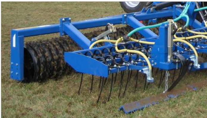
2 rows of tines with mole hill board 2 rows of 12mm harrow tines in combination with a mole hill board
