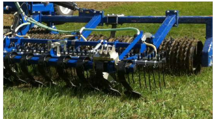
2 rows of tines with crackerboard 2 rows of 12mm harrow tines in combination with a cracker board
