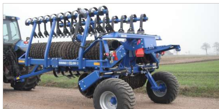
MiniMax XL with hydraulically adjustable cracker board
