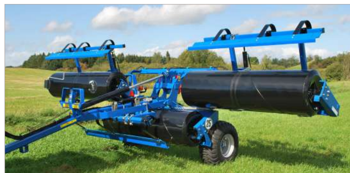
MiniMax XL Greenline model with hydraulically operated molehill board
