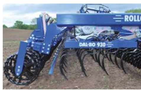
Each of the 1.55m harrow sections on the Rollomaximum XL are suspended in a parallelogram and have 4 rows of tines. Spaced at 80mm, with 300mm between each row, soil and trash can easily flow through the machine. This ensures a uniform working depth whilst providing excellent contour following across the full working width of the machine.
