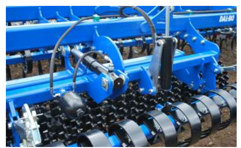
Rollomaximum XL 9.30 and 12.40 have, as standard, the front rollers mounted in a 2-D pendulum protection system.
