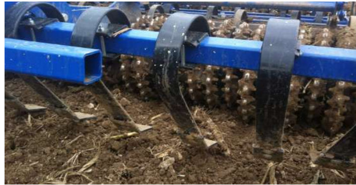
Rollomaximum fitted with a hydraulic cracker board.
