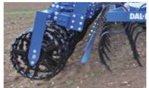
Levelling board and rear roller Between the harrow and the rear steel Crosskill roller Rollomaximum XL is fitted with a spring suspended leveling board. The board simply levels the surface so the following 50/45cm Crosskill roller can leave a fine and consolidated seedbed. Alternatively the crosskill roller can be replaced by a 45cm cage roller.
