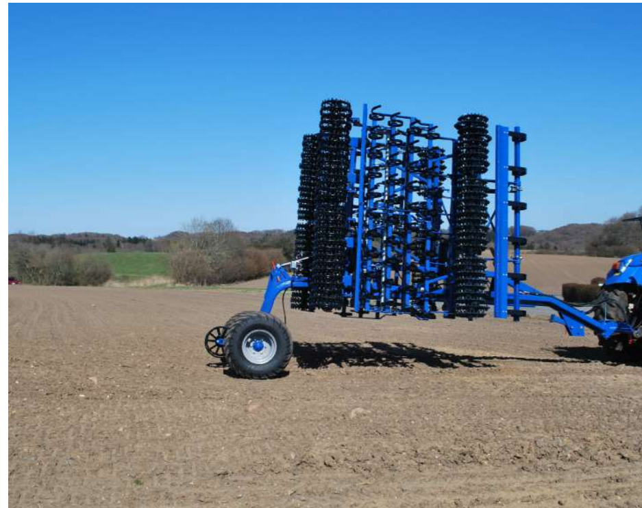
Hydraulic cracker board At the front of the 9.30 and 12.40 Rollomaximum XL is a parallel suspended cracker board. The depth is hydraulically controlled while the angle of attack is adjusted manually by spindles. On the 6.20 and 7.50 models a hydraulic leveling board or crackerboard is fitted.
