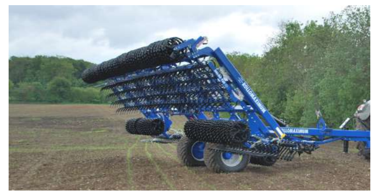
... The machine is lowered onto the ground by the wheel frame, the hydraulic pressure on the side frames is increased and the work can start.
