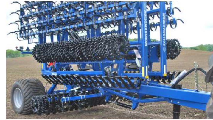
First of all the side sections are lifted clear of the transport locks..
